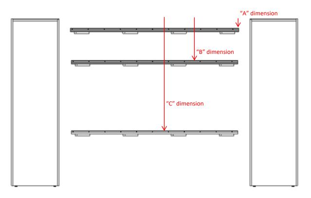
"A" Dimension – place the wall cleat up against the preassembled overhead cleat. Measure from the top of the overhead to the bottom of the wall cleat. Use this dimension from the top of the tower down to the wall location.
